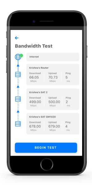
To run a bandwidth test simply select the "Begin Bandwidth Test" button at the bottom of the screen. The speed test will first run between the GigaSpire and the Internet and then will conduct a speed test between any mesh units and the GigaSpire. Results will show as a notification, update at this location, and on your main dashboard. Note: This feature is only available with a GigaSpire.
